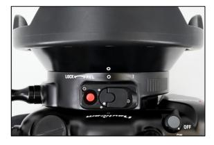
To lock the port in place, turn the port lock/release latch anti-clockwise to the original position and then flip it down.
